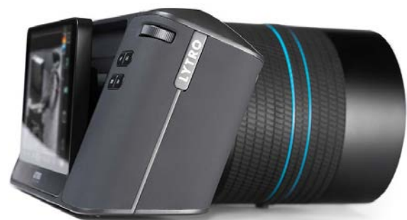
Figure 2: Lytro Illum light-field camera [4].
